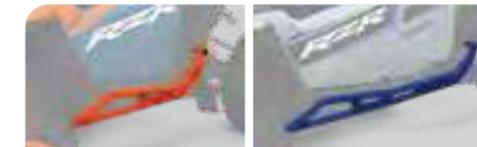
1.75" STEEL TUBE CONSTRUCTION WITH 70% THICKER WALLS, EXTENDS FROM MACHINE FOR MAX PROTECTION THROUGH ROUGH TERRAIN
